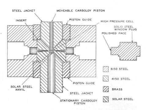
Fig. 1 Diagram of 0-53,000 atm pressure cell.
